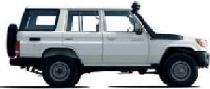
Land Cruiser 76 Series 5 door Hardtop 4.2 Diesel / 10 seater / 4x4 LHD model code: HZJ76L-RKMRS / RHD model code: HZJ76R-RKMRS
