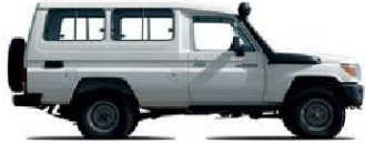
Land Cruiser 78 Series Hardtop 4.2 Diesel / 13 seater / 4x4 LHD model code: HZJ78L-RJMRS / RHD model code: HZJ78R-RJMRS
