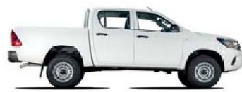
Hilux Double Cabin 2.5 Turbo Diesel D-4D / 6 seater / 4x4 RHD model code: KUN125R-DNF5HN (only available in RHD)
