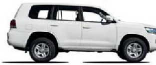
Land Cruiser 200 Series Station Wagon GX-R V6 4.0 Petrol (Unloaded) / Manual / 8 seater / 4x4 LHD model code: GRJ200L-GNMAK (only available in LHD)
